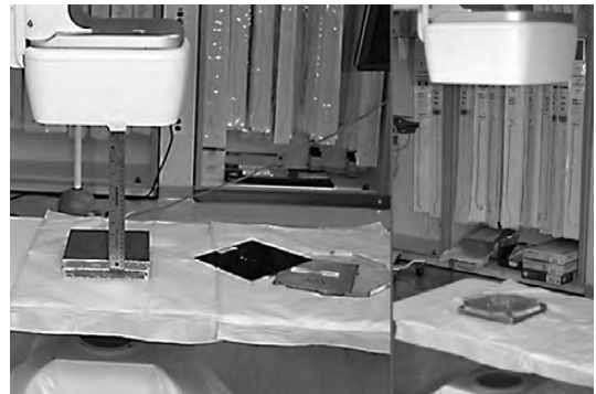
Figure 6. Representative US IQ test geometry. The test-objects are placed on the AI attenuator which is at 30 cm from the image receptor. Magnification is approximately 1.5 for this interventional C-arm. Additional HC testing is done at maximum SID (Mag. \approx 2.0 ) to further investigate the effects of the focal-spot.
